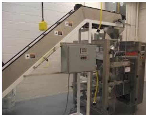
Image: Viking-Masek vertical food-grade packaging machine students use in class
